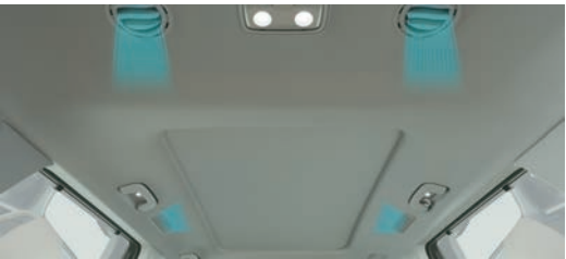
Roof Mounted Air Vents
